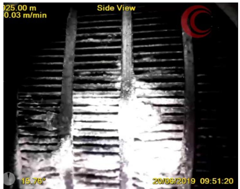
Sideview of Sand Screen showing extent of build-up
